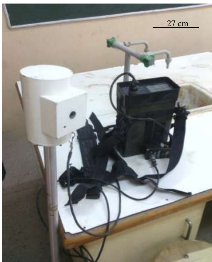
Plate III: Shows the G-856-Mag TM ProtonPrecision Magnetometer used for the magnetic data acquisition.
